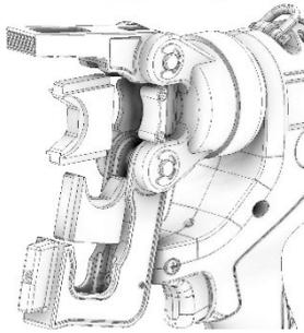
Select the dies set. Open the head and then insert the dies into the crimping head (ball headed dowel).
