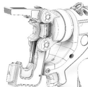
Open the head to remove the crimping connector.
