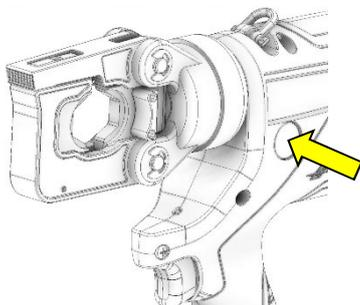
If necessary, press the emergency release trigger.
