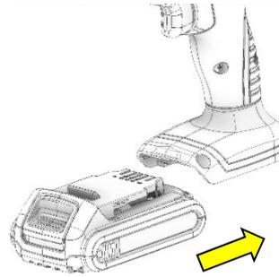
Slide the battery all the way into the tool until lock clicks.
