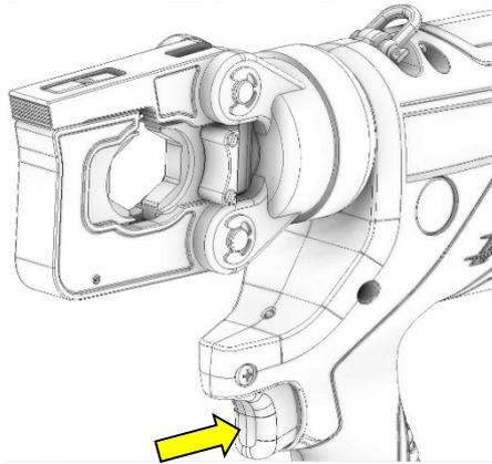
Put the connector with the cable inserted between the two dies.
