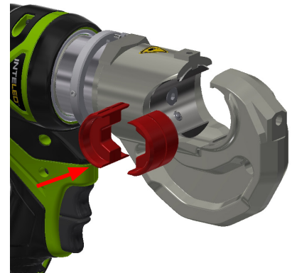
Insert the die into the crimping head.
