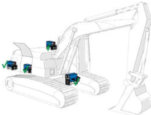
Picture 23: Location of the HG Hydraulic Generator
