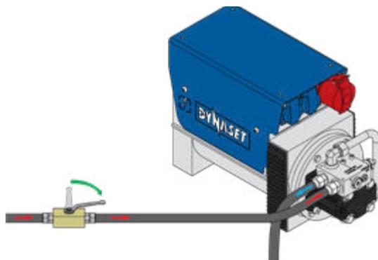
Picture 31: Starting the HG Hydraulic Generator
