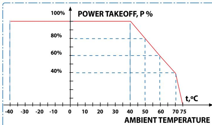
Picture 37: Power take off in higher temperatures
