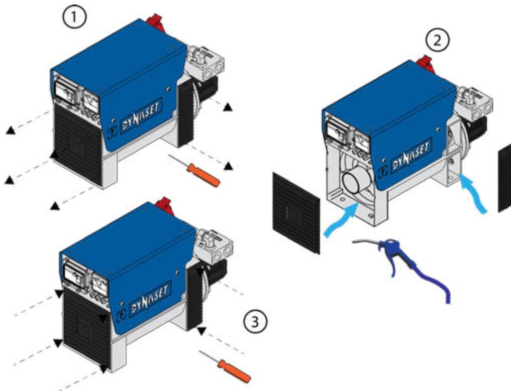
Picture 38: Cleaning the HG Hydraulic Generator
