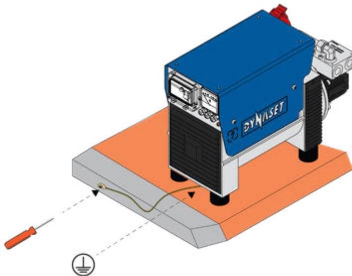
Picture 29: HG Hydraulic Generator grounding, in picture HG 6,5
