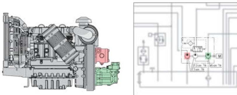
Picture 26: Base machine's pumps
