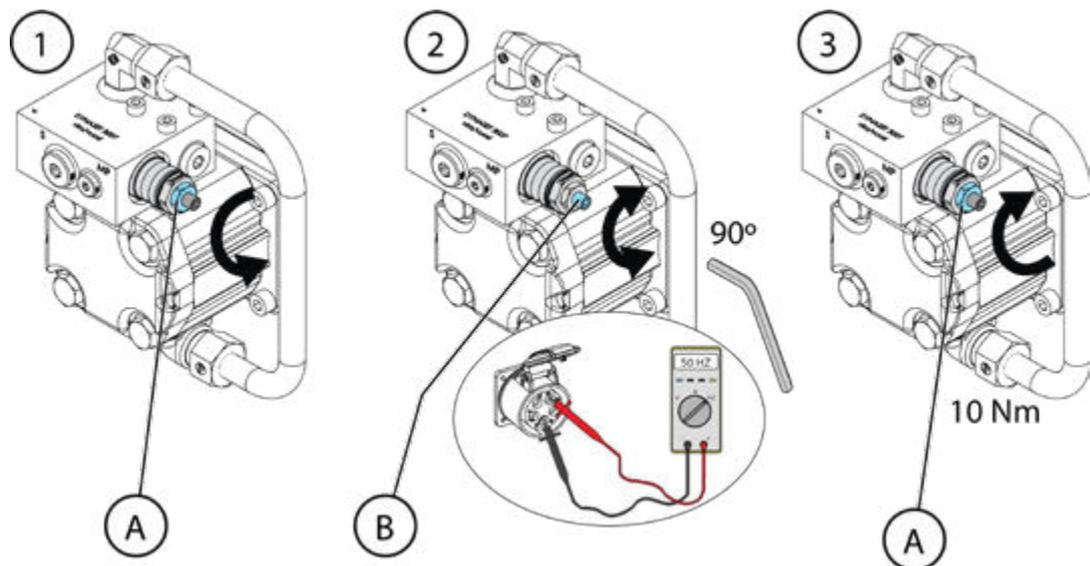
Picture 40: Adjusting the RMP-cartridge
