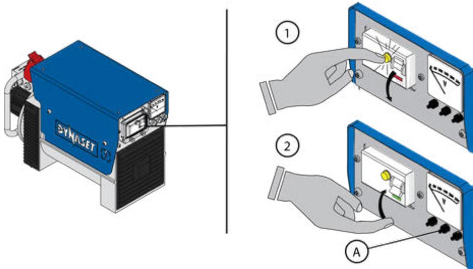
Picture 39: Testing the residual current device
