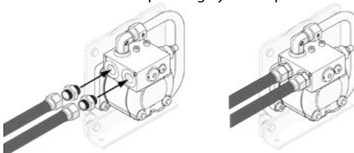
Picture 24: Installing hydraulic hoses
