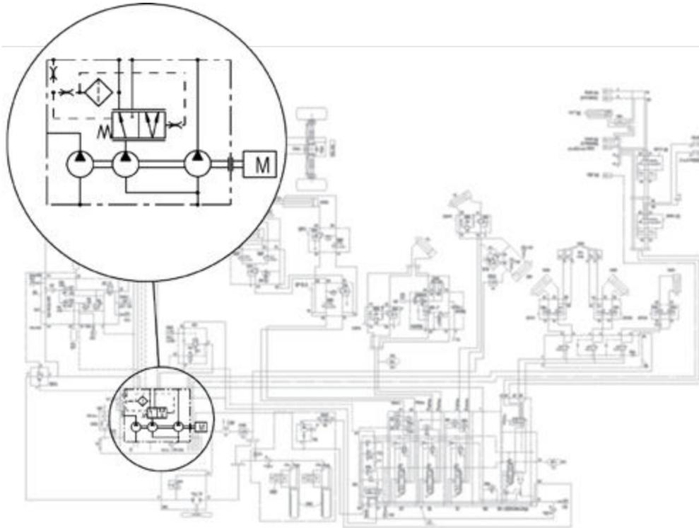
Picture 18: Hydraulic system with fixed displacement pump
