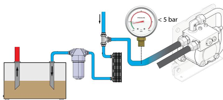
Picture 27: Return line (T) pressure must be under 5 bars.
