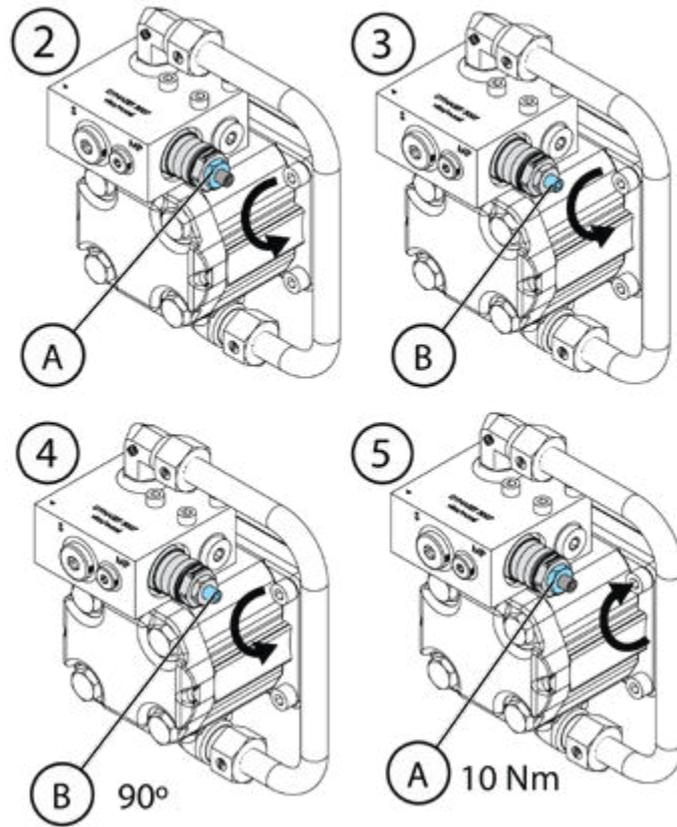
Picture 42: Adjusting the RPM-cartridge without installation valve 2
