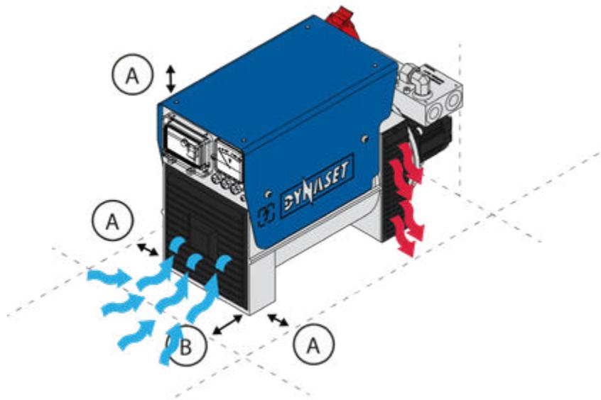
Picture 28: Placement of the HG Hydraulic Generator with sufficient room and ventilation
