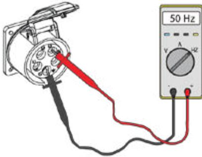
Picture 32: Metering frequency from the socket
