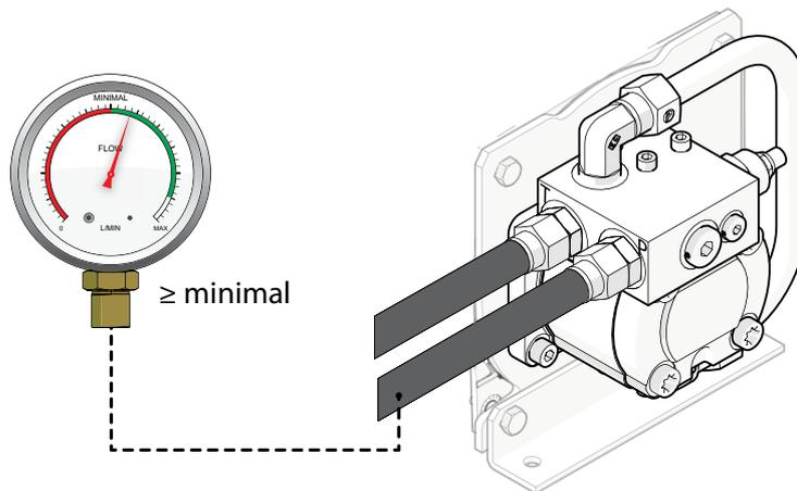
Picture 25: P-line operational hydraulic flow
