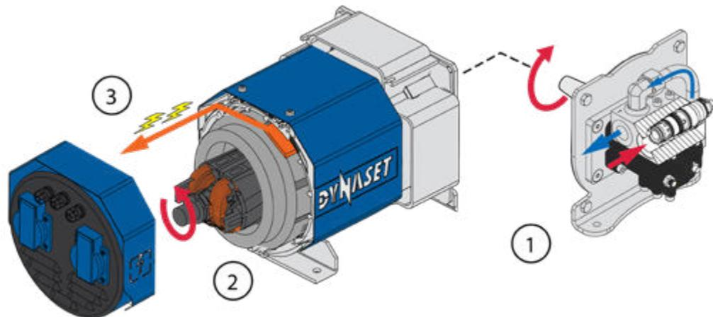
Picture 11: HG hydraulic generators operating principle
