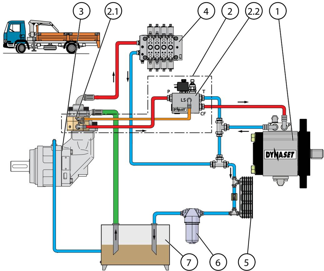
Picture 19: Connection figure for hydraulic system with fixed displacement pump
