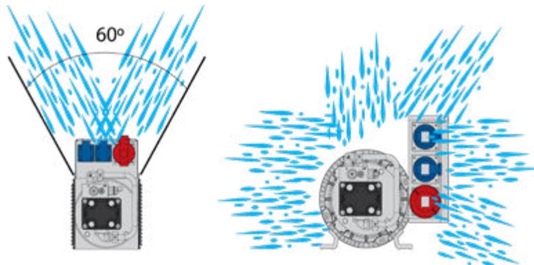
Picture 30: IP23 and IP54 positioning
