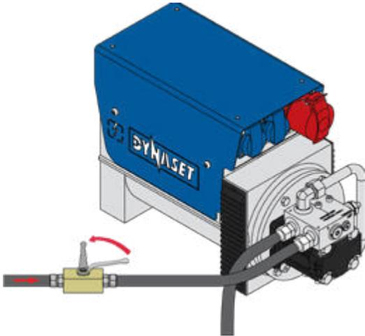
Picture 36: Stopping the HG Hydraulic Generator
