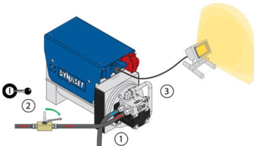
Picture 35: Connecting load to the HG Hydraulic Generator
