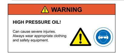
The pressure in hydraulic circuits is considerably high. Therefore the condition of your equipment are to be kept under constant observation. All couplings, valves and hoses are to be kept tight and clean. Leaks in the hydraulic system must be repaired immediately to avoid injuries caused by high pressure and oil blowouts.
