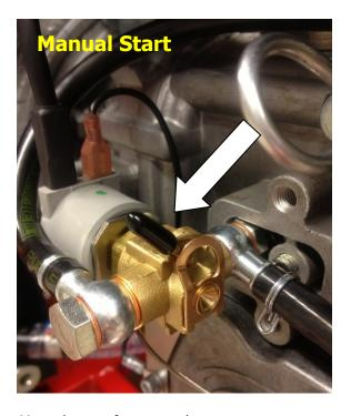
Manual start of powerpack. Lever is pushed away from the engine block. Engine cannot be turned on and stopped by turning ignition key. Use recoil start.
